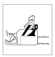
6 The way the chain brake is triggered, either manually or automatically, depends on the force of the kickback and the position of the chain saw in relation to the object that the kickback zone of the bar strikes.
